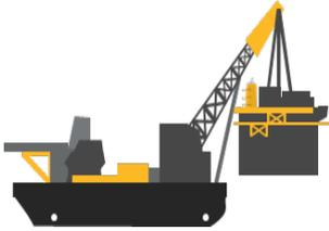
**Application:** Used for installation of jackets (for WHPs and CPPs) and topsides (for WHPs).
